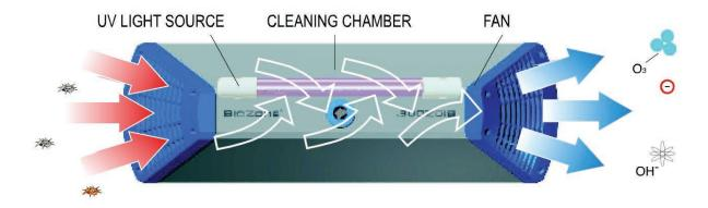
\*Air does not need to pass through the chamber to be purified due to the unit transmitting ozone, photoplasma and negative ions.
